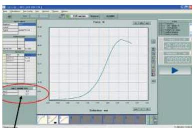
**"Mini-VAL" SPECIAL DESIGN:** To perform physical-mechanical tests on egg containers (**Flexion - Tensile and Compression**) with a single top load cell and easy-to-use interchangeable test tools.
