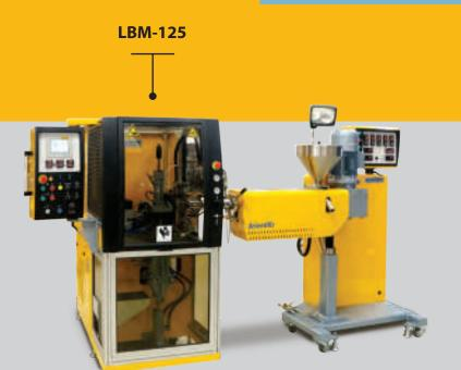
Fully automatic hydraulic laboratory Blow Moulding attachment with LCD touch screen controls
