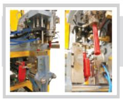
Discharge pins will hold the bottles after blowing for one cycle to allow additional cooling before it is automatically dropped into the discharge chute where it will exit out at the left side of the machine body. The strip is heated by a low Voltage, high Ampere supply from a built in power unit.
