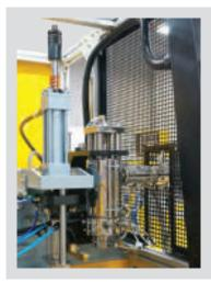
The extruder can be seen on the far right of the picture feeding into the die. The Blow pin unit, hydraulic cylinder and piston (pin) are on the left.
