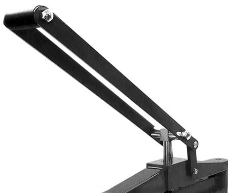
The lever is easy to operate, it has a length and a push system with a small force to cut quickly. They have the threaded end for easy disassembly when necessary.
