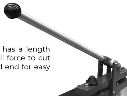
The Model MP-15 and MP-25 presses, due to their long cutting length of 300 mm, use a special double lever system, requiring very little effort to cut the samples.
