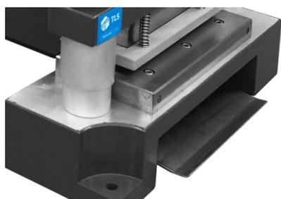
Model MP-10, MP-1010, MP-15 and MP-25 presses are equipped with an inclined platform underneath the blades so that the already cut samples can slide and in this way they can be easily extracted.
